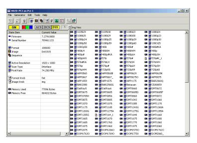
The left pane displays basic properties of the format currently being used by the generator. For detailed format information, click the licon. Use this detailed view to sort formats by different properties.
